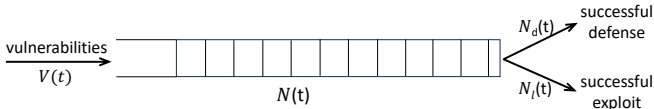
Fig. 1. Attack surface modeled as a queueing system. Vulnerabilities arrive via V(t) and depart through competing defense (patching) and exploit processes.
